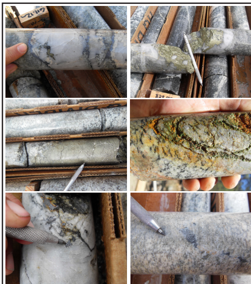
Photos of common mineralization styles and textures. Clockwise: 1) Qz-cp-py-mt/mo veins with thick molybdenite envelopes. 2) Thick qz-cp±(mo-py) vein. 3) Native copper and copper oxide is visible within fault related fractures near the top of hole CB-13-07. 4) Sulfosalt-bearing vein within the Bradshaw granite, near the bottom of hole CB-13-03. 5) Sooty chalcocite within wide quartz vein. 6) Zone of intense QSP alteration within CB-13-03, resulting in very high sulfide (py>>cp) content.
