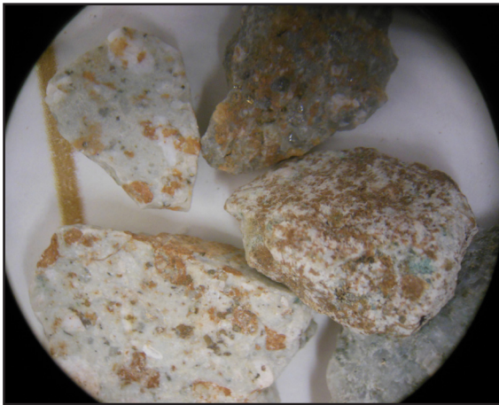
Cuttings from historic drilling showing multiple sericitized porphyries and Cu-ox after sulfides
