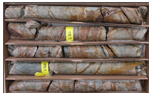
Styles of mineralization encountered in drilling. Shown are quartz-limonite-chalcopyrite (porphyry-style) veins cut by vuggy quartz-limonite veins (epithermal-style) intersected in drill hole IO-1.
