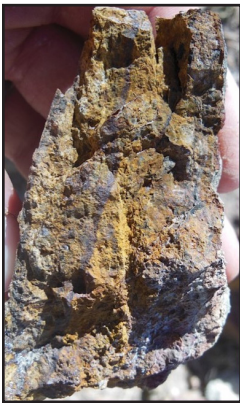
Decalcified Joana limestone cut by sulfide veinlets contains anomalous As (>1,000ppm), Sb (>100ppm), and weakly anomalous Au.
